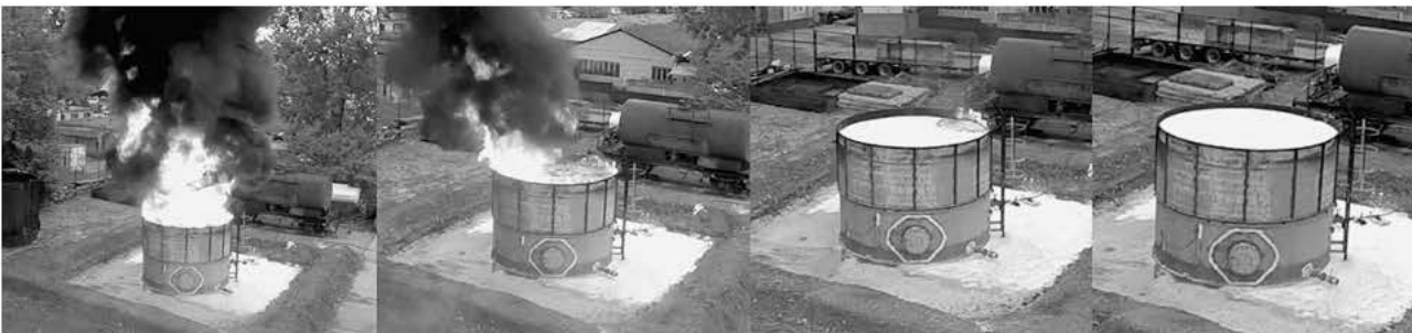
FIGURE H.3.2(c) Extinguishing Sequence, FFF, Subsurface Injection.
