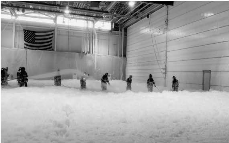
FIGURE A.7.6.2.3(c) Firefighters Sweeping 6 ft (1.8 m) Wands in a 180-Degree Motion Searching for Anything Hidden Beneath the Foam.
