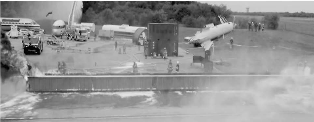
FIGURE H.3.2(b) A 98 ft (30 m) Flow Test Approaching Full Extinguishment.
