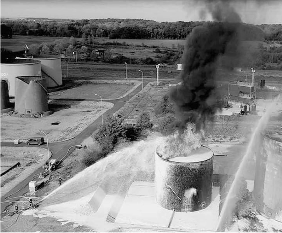
FIGURE H.3.2(a) From LASTFIRE: FFF — 36 ft (11 m) Tank Fire Testing.
