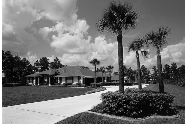
▲ FIGURE A.17.1.9.2(a) Planting Islands Offer Exposure Protection, Preserve Aesthetics. (Courtesy of Firewise Communities Program. Photo by G. Johnston.) [1140:Figure A.24.3.5.2(a)]
