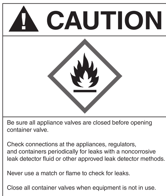
N FIGURE 50.8.5.6 Appliance Caution Plate. [96:Figure 17.5.6]
