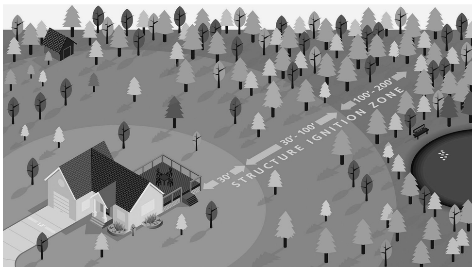
△ FIGURE A.17.1.8 The Structure Ignition Zone. (Source: Firewise Communities Program.) [1140:Figure A.24.3.4]
