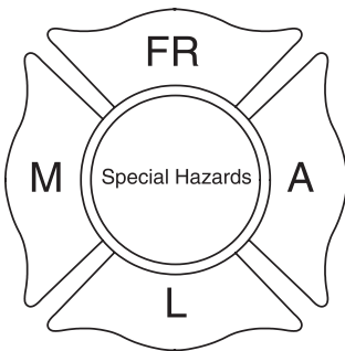
FIGURE C.1.2.3 Sample Sign for Firefighter Safety Building Marking System.
